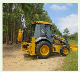
Figure 2.3: Tractor Loader Backhoe
